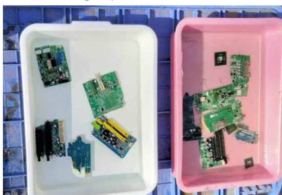
Figure 1: The formation of e-waste leachates using non-acidic static process using two personal computer mother boards (PCMB) immersed in lake water and incubated for 30 days.
