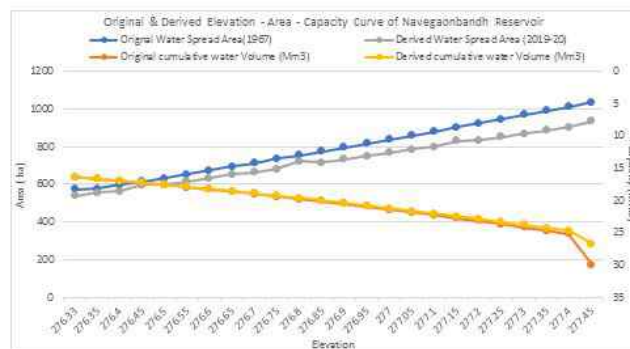
Fig. : Original & Derived Elevation - Area - Capacity Curve of Navegaonbandh Reservoir, showing, the average rate of loss of capacity is computed to be 0.062 Mm 3 (0.20%) per year during 1967 to 2019-20.
